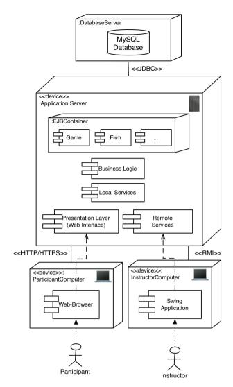
Fig. 4. Deployment diagram.
