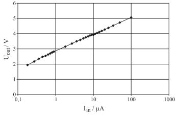
Figure 4. Response curve of logarithmic transimpedance amplifier
