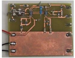
Figure 3. PCB circuit of linear transimpedance amplifier
