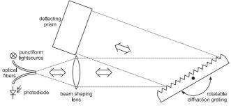
Figure 1. Optical setup of OSA
