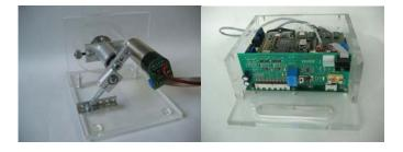
Figure 4. Mechanism and DSP-2 controller
