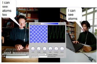
Figure 1. Friction mode of the nanosimulator. Two students observing stickslip phenomena between a tip and an ultra flat NaCl surface. The simulation window contains several wheels for parameter settings as well as measurement results including visualizations.
