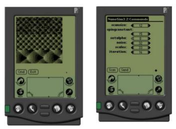
Figure 4. NanoMobile remote steering interface on a PDA. Left: View of an observed surface with atomic resolution. Right: List of gauges to view and adjust experiment parameters.
