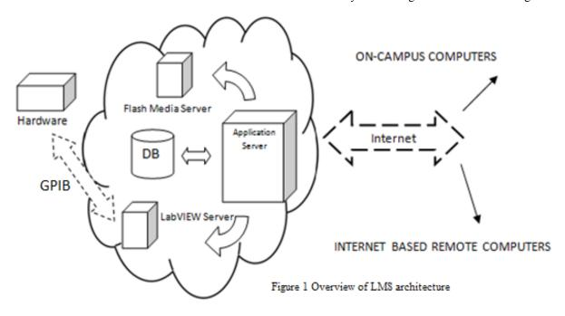
These interfaces are built using the web development tool of NI LabVIEW 2009. The devices are connected and controlled by using the interface and their corresponding drivers.
