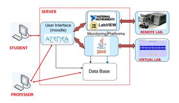
Figure 1. Remote laboratories and Virtual Laboratories are connected to the server through a software platform: Java or Labwiew. Atenea is the user interface (UPC Digital Campus).
