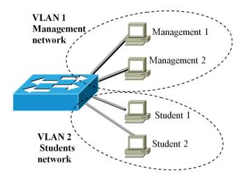
Figure 3. Two VLAN networks in a single switch.
