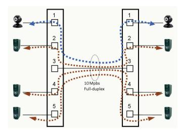
Figure 4. Schema used to obtain congestion in a network link. Both switches are connected trough port 3. The computers on port 1 of each switch make a videoconference enconded with 4.5 Mbps. The other computers transfer files on both senses.
