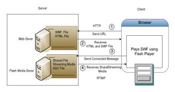
Figure 2. Procedural sequence steps in general connecting and displaying share and streaming media.
