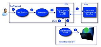
Figure 4. Block diagram of the new security model
