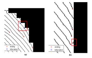
Figure 7. Results of the extraction of minutiae points: (a) Detail of the false bifurcations extracted; (b) Detail of false ending extracted.
