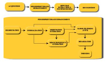
Figure 5. Block diagram of the fingerprint identification system
