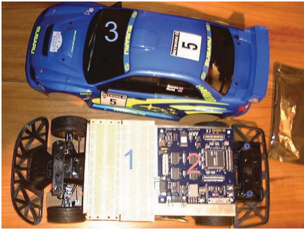
Figure 1. Car model modified to include a breadboard (1) and a printed circuit (2) without the plastic cover (3).
