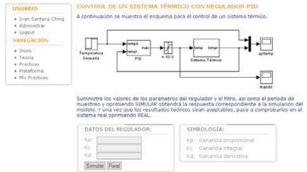
Figure 3. Web Page of thermal system practices with regulator PID.
