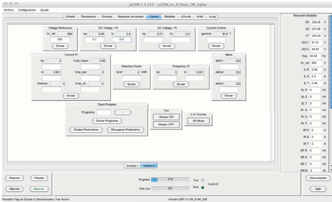
Fig. 7. Controller screen where the tuning of the controller constants can be done.
