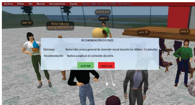
Figure 4. Teachers' Recommender system in action. The Evaluator Object displays the recommendation in the teacher's view centre. Information collected from the students' questioning objects is used by the recommender to guide teacher's activity in real-time.
