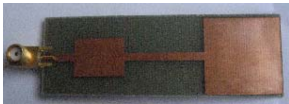
Figure 4. Example of a 2.4 GHz patch antenna.
