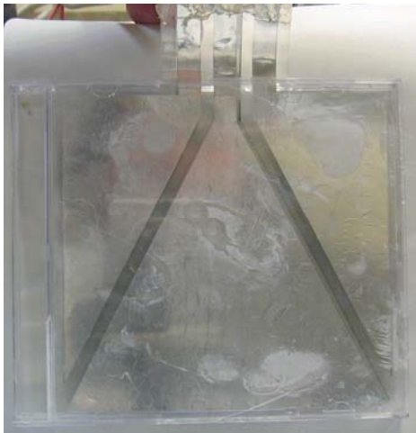
Figure 2. Flat capacitive sensor of triangles based on a CD box.
