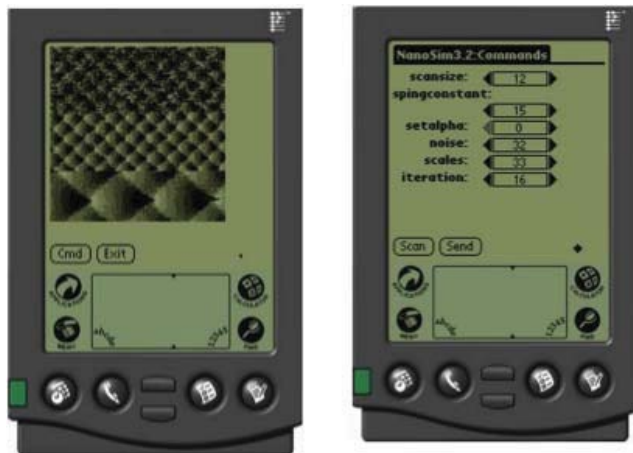
Figure 4. NanoMobile remote steering interface on a PDA. Left: View of an observed surface with atomic resolution. Right: List of gauges to view and adjust experiment parameters.
