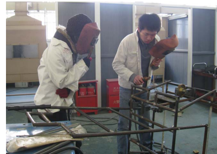
Figure 6. Students are Welding the chairs in workshop
