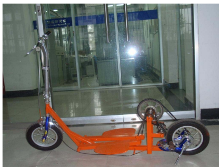
Figure 4. A skateboard bicycle manufactured by students
