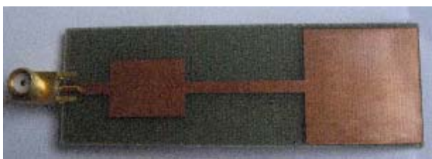
Figure 4. Example of a 2.4 GHz patch antenna.
