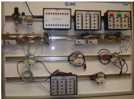
Figure 5. A two cylinder workbench used in practical lessons.
