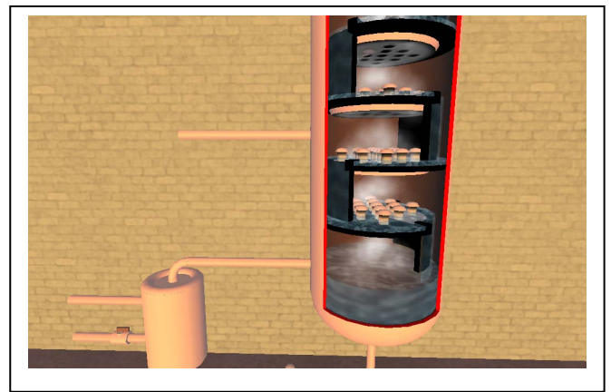
Figure 6. A virtual distillation column demonstrating visualisation capabilities inside the virtual world. Shown are the Column internals including the trays through which vapour rises contacting the liquid falling down on top of the trays.
