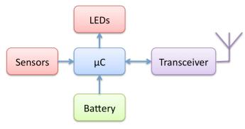
Figure 2. Block diagram of a basic WSN node.
