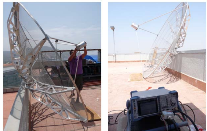
Figure 12. Assembly of the horn at the parabolic focal point and tests.
